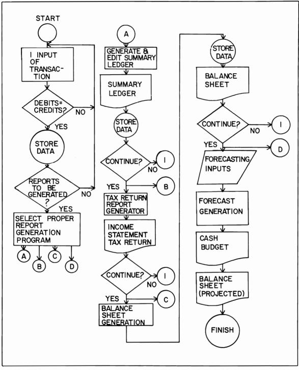
Fig. 2-2. A flowchart for an accounting system program.
